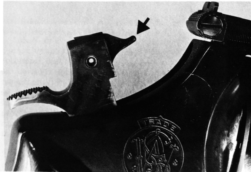
Figure 1-2A. The firing pin point strikes the primer and fires the cartridge. (Smith and Wesson revolver.)
