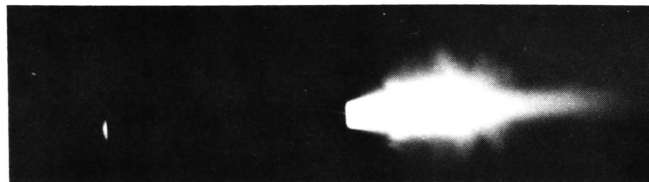
Figure 1-3. A Colt four-inch barrel revolver firing a .357 Magnum primer in an empty cartridge case. The flash is visible (left) in the gap between the front of the cylinder and the rear of the barrel throat. Note the amount and intensity of the flame as it bursts from the muzzle (right).
