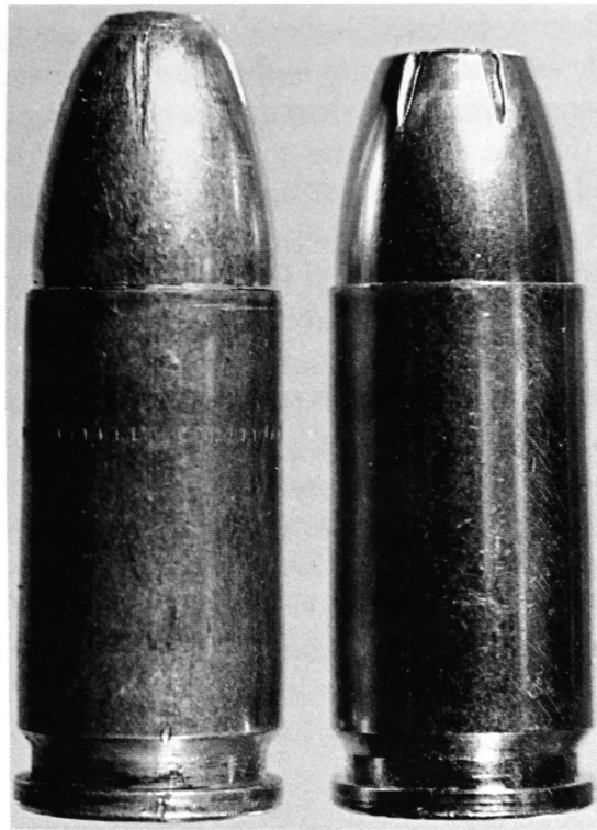
Figure 1-2. Two variations on the 9mm cartridge. On the left is a round nose, jacketed, soft point cartridge. On the right is a truncated nose, jacketed cartridge.
