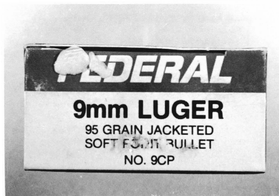
Figure 1-11. Federal #9CP 95-grain JSP. Not recommended for general law enforcement, but this ammunition could have application to special situations. Lightweight bullet tends to go to pieces upon impact (Average velocity 1320 fps, Variation in velocity 49 fps).
