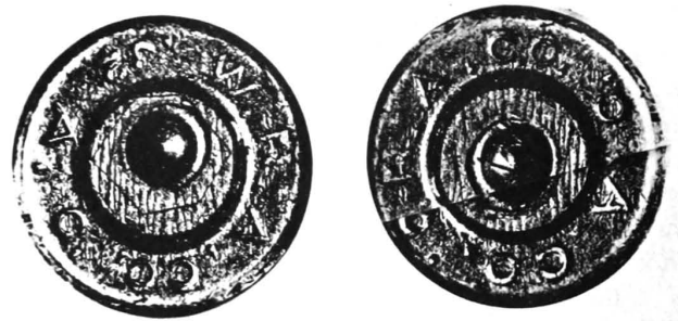
Fig. 14. Method of interchange. (Applied to photos in Fig. 26.) Left: A portion of the photo of the Lowell Test Shell has been cut out and placed on the Evidence Shell. Right: A portion of the photo of the Evidence Shell has been placed on the upper part of the Lowell Test Shell.
