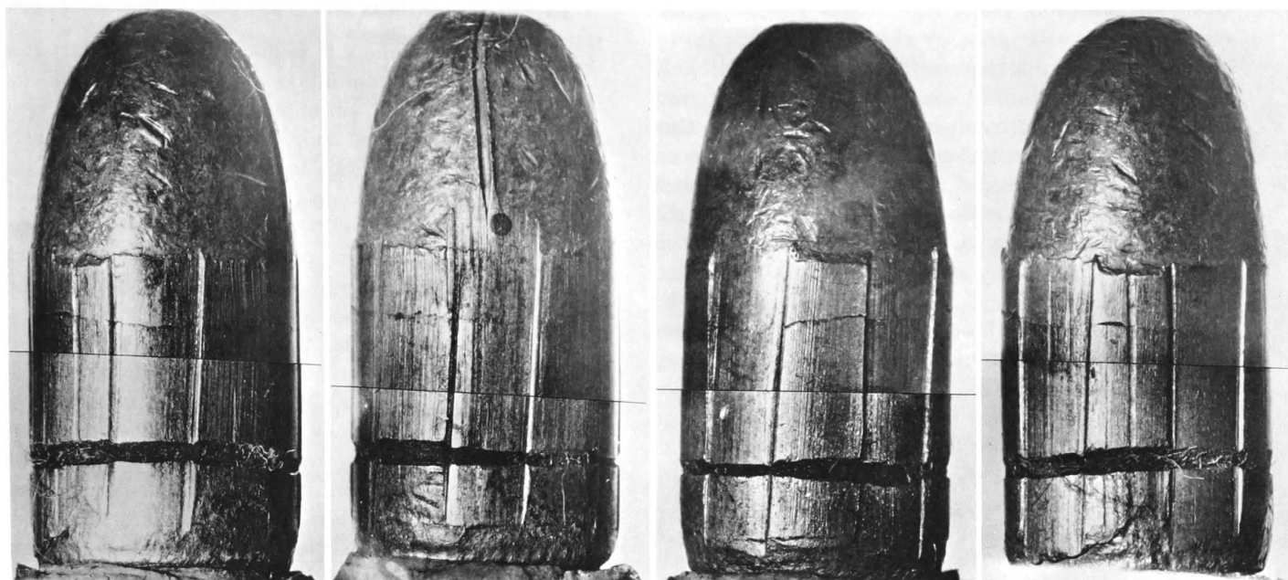
Fig. 11. Comparison camera photos showing four matchings found on a pair of bullets fired from a .38 cal. S & W revolver.
